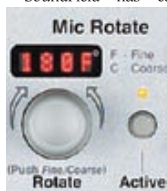
The Rotate controls on the DSF-2 decoder allow the mic to be 'turned' without physically altering its position, by altering the balance of the B-Format signals with respect to one another.
