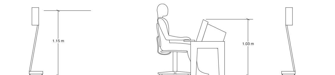
Figure 2 : Side view of loudspeaker configuration (side speakers omitted for clarity; to scale)
