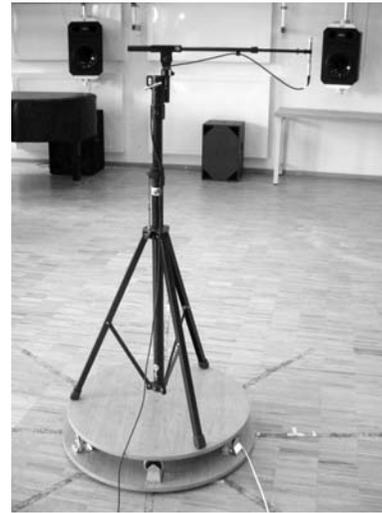
Figure 3: The microphone on the rotating table .
