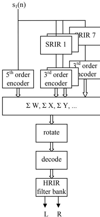
Figure 2: System for one static sound source.
