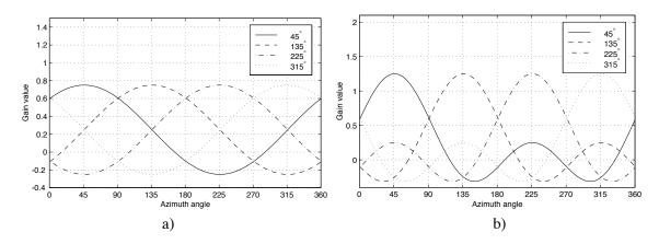
Figure 3.2: Gain factors for a quadraphonic loudspeaker setup calculated with a) first-order Ambisonics b) second-order Ambisonics.
