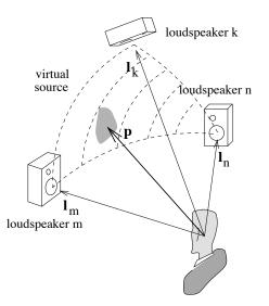
Figure 3.3: A loudspeaker triplet forming a triangle formulated for three-dimensional vector base amplitude panning (VBAP).
