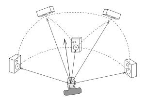
Figure 3.4: Triplet-wise amplitude panning with five loudspeakers.
