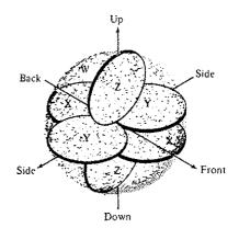
HE CALREC CM 4050 Soundsield Microphone consists of four hypercardioid capacitor capsules arranged in a regular tetrahedron so as to detect the soundsield at the surface of the sphere. The signals derived from the four apsules are known as A Format signals.
