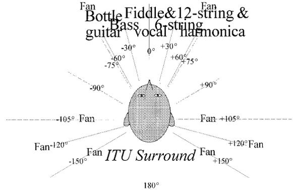
Fig. 4. Contrasted with PanAmbio, ITU 5.1 "relocates" quintet+fans by angular distortion (although less than two-speaker stereo). Original angles indicate sounds recorded at  $\pm 75^\circ$  are heard at  $\pm 30^\circ$  and are superimposed within the band. If precision localization is not essential to a recording, ITU 5.1 may be quite acceptable.
