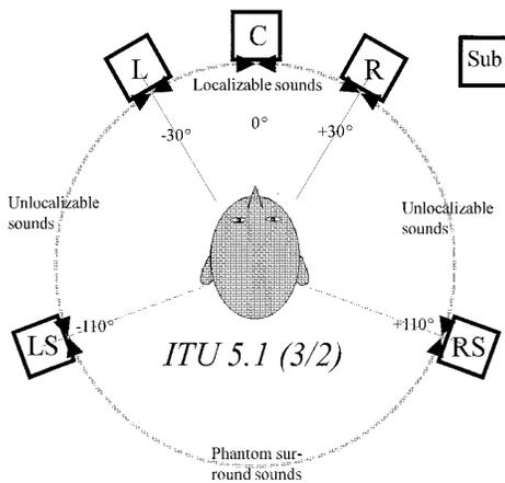
Fig. 1. ITU 5.1 (3/2) standard speaker placement creates five sets of phantom images, one between each pair of transducers, that surround the listener and makes it superior to stereo in “realism.”
