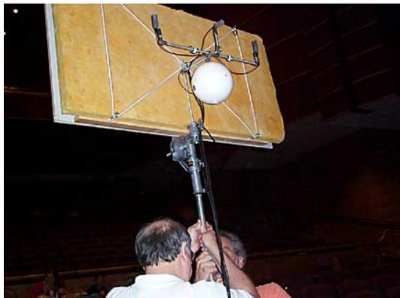
Fig. 6. Hoisting OCT and prototype Ambiophone microphones in the 1,000-seat opera house. Microphones are Schoeps CCM-series.
