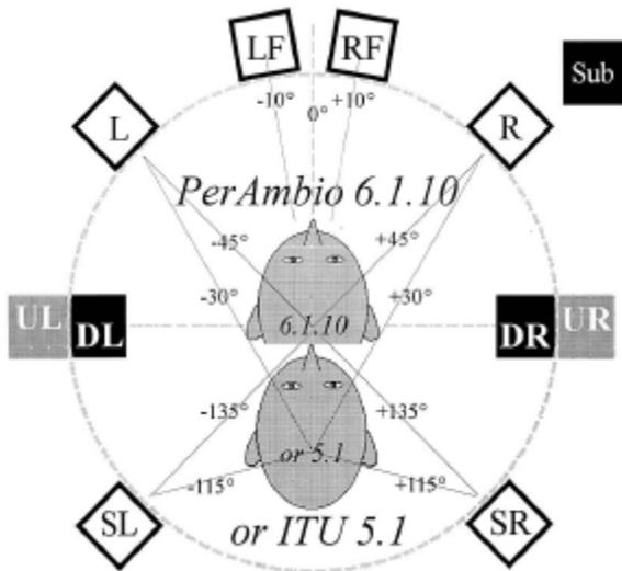
Fig.8 – Compatible PerAmbio 6.0.10 spherical surround hybrid of Ambisonics + Ambiophonics accommodates audiences up to six. For 5.1, viewers sit back 26% of the speaker diameter, where the angles meet ITU standards (DSP changes levels/delays). For 3D music appreciation, one or two listeners sit at the focus of 10 speakers.
