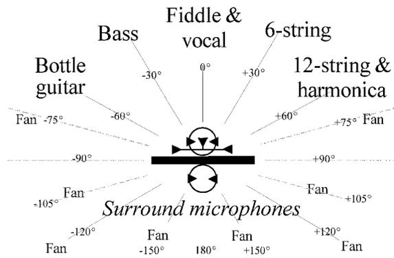
Fig. 5. Microphone arrays contrast two 360° reproduction methods. PanAmbio uses twin spheres with baffle. For ITU 5.1, OCT uses two supercardioids facing  $\pm 90^\circ$  and cardioid facing front. Simultaneous recordings of guitar quintet + fans, opera, brass quintet, string quartet, marching bands, and "Perambulating 360°" azimuth test were authored to companion DTS-encoded CDs for evaluation [8].
