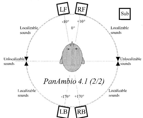
Fig. 2. PanorAmbiophonic 4.1 (2/2) speaker placement turns stereo “inside out,” creating accurate images outside pairs of transducers. It can serve as a benchmark of quality for, or alternative to, ITU 5.1.
