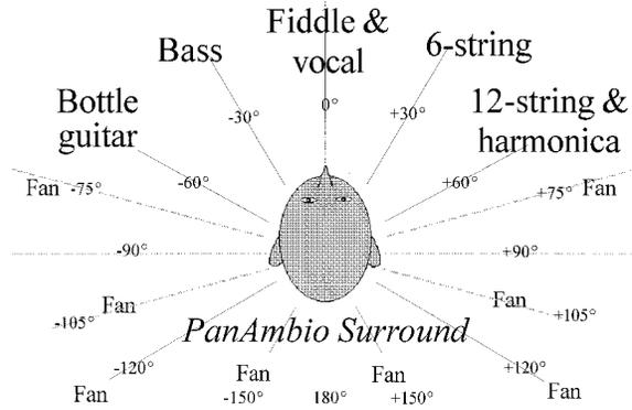
Fig. 3. PanAmbio 4.1 (2/2) reproduction localizes sources accurately within  $\pm 5^\circ$ , virtually duplicating the recording session directions in Fig. 5 below. Guitar quintet and fans are placed as shown for experiments that contrast two 360° reproduction methods. Multi-channel surround sound is more "realistic" by localizing both front stage instruments and sounds from around and behind, including antiphonal voices, audience participation, and ambience.
