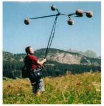
This is Mr.Florian Camerer of ORF(Austria Broadcasting Corporation). He is recording field locations with 5-ch microphone array. On his shoulder are three 2-ch portable DAT recorders for surround sound recording, with synchronized timecodes. This requires physical strength. Mr.Florian Camerer's 5ch human miking is based
