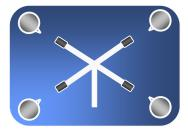
This cross bar is called IRT-cross. Four microphones are placed at the corners of a 21-cm-square. These are CCM-4 Schoeps cardioid microphones.
