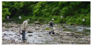
This is a 5-m-square microphone array. Four CCM-4 Schoeps cardioid microphones are placed at the corners of a 5-m-squre.
