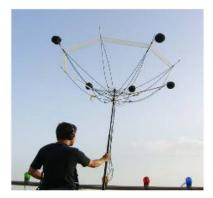
An audio mixer at NHK ordered a craftsman to make a fiberglass umbrella-shaped microphone boom pole. He put five CCM-2 Schoeps omni-microphones at each end of the ribs of the umbrella-shaped boom pole. Each microphone distance is 80 cm.
