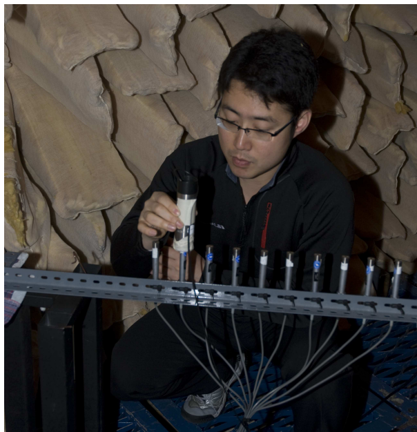
FIGURE 8.16: Microphone array calibration, performed by Dr. Mincheol Shin.
