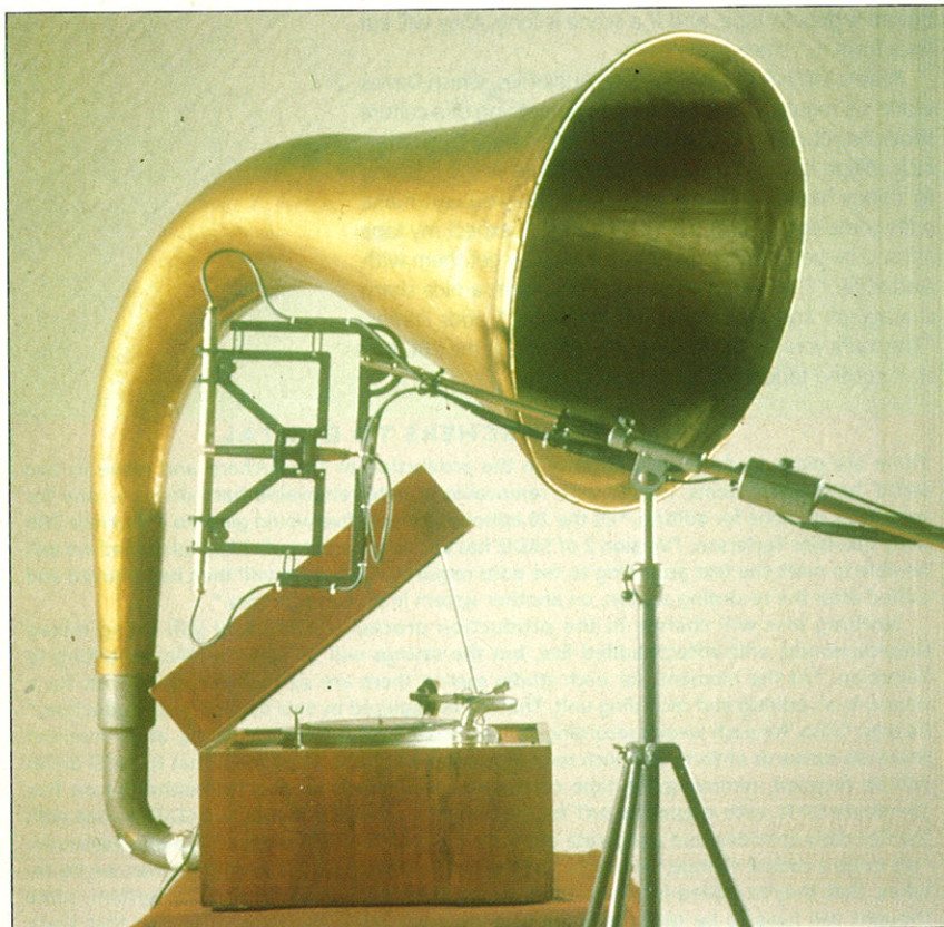
The specially-designed Nimbus Halliday Ambisonic Microphone array, shown with an EMG c1935 "Expert" Gramophone.
