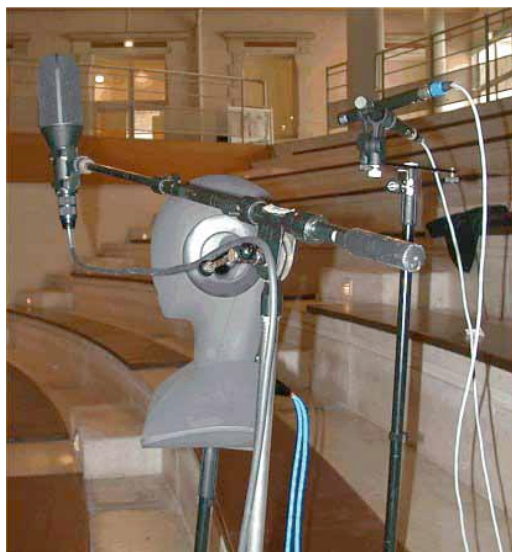
Figure 1. Simultaneous recording of the 3 techniques: artificial head for transaural reproduction, Soundfield microphone for ambisonics reproduction and ORTF pair for stereophony.
