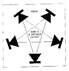
The Ambi-5 Decoder: The Ambi-5 set in five pointed star array, was very successfully used by the Cure on their USA tour, using five massive sound reinforcement arrays. This layout has the advantage of offering a natural stereo pair to the front of the system. The decoder generates five balanced line level feeds with a loudspeaker angle separation of 72 degrees. Its rotated output produces an offset of 36 degrees. Cascading two Ambi-5s will create a 10-speaker matrix at 36 degree intervals.
