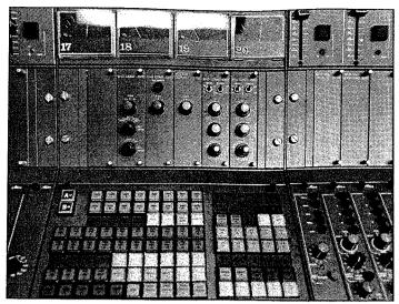
The transcoding from the mixing format to the transmission format is effected in the module marked B-C. To the right of this is a set of decoders which allow vectorial display of the sound field on an oscilloscope and aural indication on two different sets of loudspeakers, one of which is set in the vehicle. The PPMs can be switched to either B-, C-or D-format signals.
