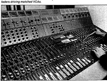
On the right-hand side of the nearer set of monophonic channels are the special 3-channel groups. These groups have balance attenuators at the top of the modules which provide equal amounts of coarse attenuation in each of the three channels; the continuously variable control is achieved with the
