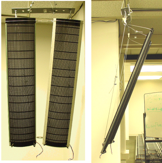
Figure 8: 9-by-32-inch curved electrostatic panels made by MartinLogan, Inc. and suspended by a cable and truss assembly
