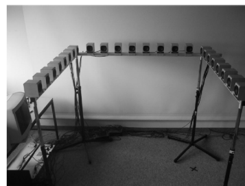
Figure 28: Small-scale wave field synthesis playback configuration
