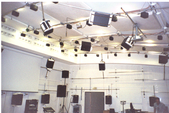
Figure 26: 32-channel hemispherical playback system at the Institute of Electronic Music and Acoustics of Graz, Austria
