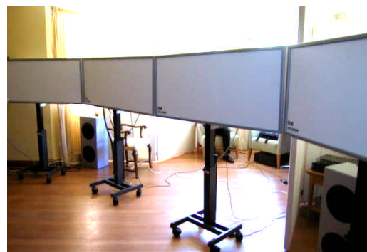
Figure 30: An array of 8-channel multi-actuator panels for wave field synthesis
