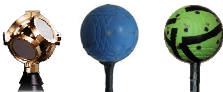
Figure 2: Soundfield microphone (left) composed by four coincident cardioids sensors. Second order ambisonic microphone prototype (middle) composed by 12 sensors positioned in dodecahedron configuration. Fourth order ambisonic microphone prototype (right) composed by 32 sensors positioned in pentaki dodecahedron configuration.
