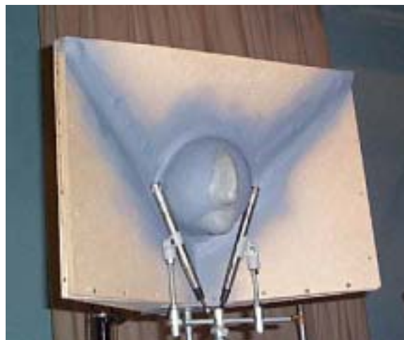
Fig. 2 Ambiphone prototype by Robin Miller before placement of omni capsules within the head
