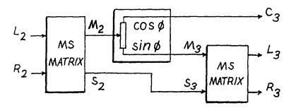
Figure 6. Form of  $3 \times 2$  decoder for three-loudspeaker reproduction of two-channel stereo using sine and cosine gains dependent on an angle parameter  $\phi$ .
