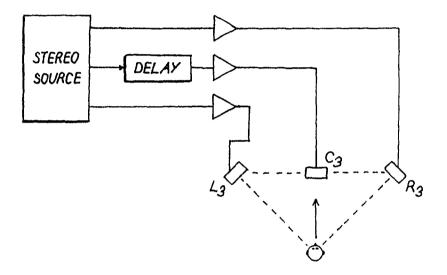
Figure 2. Use of time delay to compensate for unequal distances of loudspeakers from an ideally-situated listener.
