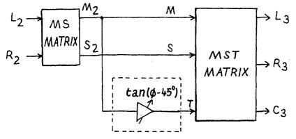
Figure 13. Version of the  $3 \times 2$  decoder of fig. 6 implemented in MST form using a synthetic T channel; this is only an approximation to the results of fig. 6, but the approximation is very good for  $|\not p-45^{\circ}| \leq 15^{\circ}$
