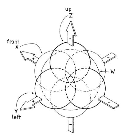
Figure 11. Polar diagrams of the B-format signals W (ommidirectional) and X, Y, Z (figure-of-eight with peak gain  $\sqrt{2}$  = 1.4142) in 3 dimensions.
