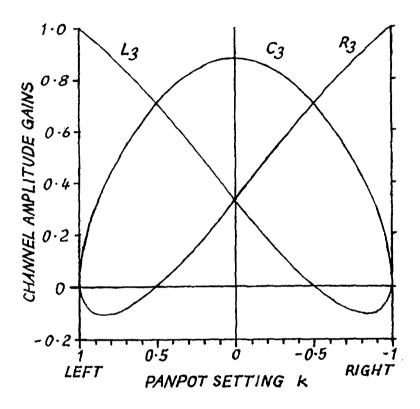
Figure 3. "Optimum" 3-channel panpot law gains for 3-loudspeaker stereo feeds L<sub>3</sub>, C<sub>3</sub> and R<sub>3</sub>, ensuring consistency of different localization cues and minimizing geometric image distortions for noncentral listeners.
