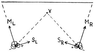
Figure 10. Illustrating the "splaying out" of the two stereo microphones, with  $M_L$  and  $M_R$  pointing at the edges of the stage, for a sound stage wider than the microphone spacing.
