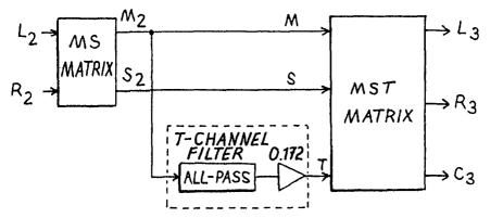
Figure 12. Psychoacoustically optimized 3 x 2 decoder of fig. 7 implemented as an MST decoder with a synthetic T channel produced by filtering the M signal; adapted from fig. 14 of ref. [28].
