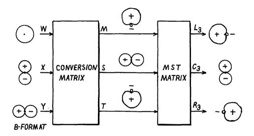
Figure 15. 3-Loudspeaker decoder for B-format input, using a conversion matrix (as in eqs. (12)) from B-format to MST signals and an MST matrix to produce loudspeaker feed signals, showing the polar diagrams of the signals.
