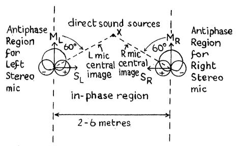
Figure 9. The use of a spaced pair of one-point stereo microphones, each of which is assymmetric, to cover a broad direct-sound-source stage. The gains of the  $S_L$  and  $S_R$  figure-of-eight microphones should ideally be such that a central sound source X in the stage is picked up as a central image, with equal channel gains, by both stereo microphones. Adapted from ref. [22].
