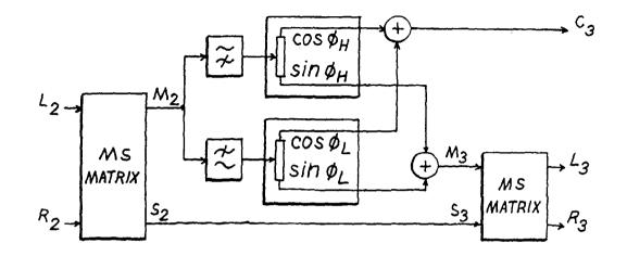
Figure 7. Frequency-dependent version of the 3 ×2 decoder of fig. 6, using low and high pass filters preceding different values,  $\phi_{\rm L}$ and  $\phi_{\rm H}$ , of the decoder parameter  $\phi$  at respective lower and higher frequencies around 5 kHz. Recommended values are  $\phi_{\rm L}$  = 35.26° and  $\phi_{\rm H}$  = 54.74°.
