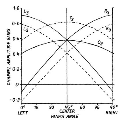
Figure 8. Channel gains for three loudspeakers L<sub>3</sub>, C<sub>3</sub>, R<sub>3</sub> when a constant-power sine-cosine two-channel panpot is fed to a psychoacoustically-optimized  $3 \times 2$  decoder. Chained lines: low frequencies below 5 kHz, with  $\phi = 35.26^\circ$ ; solid lines: high frequencies above 5 kHz, with  $\phi = 54.74^\circ$ .
