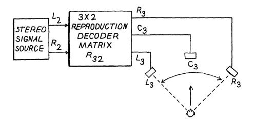
Figure 5. The reproduction of a 2-channel stero source via three loudspeakers, using a  $3 \times 2$  psychoacoustic decoder.
