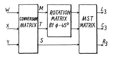
Figure 16. Use of frequency-dependent rotation matrix by angle  $\phi$ -45° in the M and T signal paths in the decoder of fig. 15. Typically,  $\phi = 35^{\circ}$  below 5 kHz and 55° above 5 kHz.
