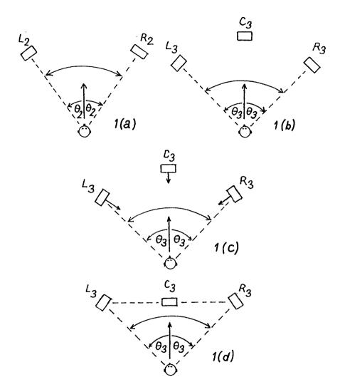
Figure 1. Two- and three-loudspeaker stereo layouts. 1(a) two loudspeakers. 1(b)-1(d) three loudspeakers. 1(a)-1(c) loudspeakers equidistant from ideally situated listener. 1(c) & 1(d) toed-in outer loudspeakers.
