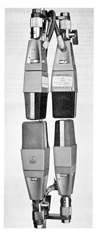
Fig. 1 - Coincident cardioid microphone array
