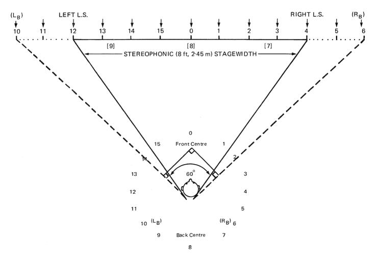
Fig. 4 - Theoretical 'equi-spaced' stereo presentation of quadraphonic sources
