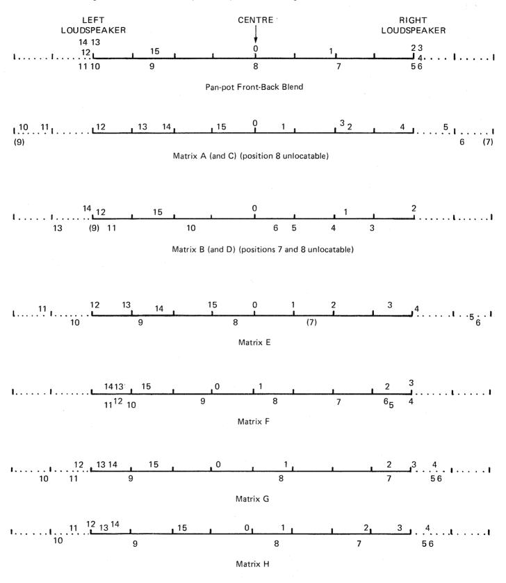
Fig. 6 - Subjective image positions – matrix stereo (pan-pot material) Bracketed figures indicate positions found difficult to locate Thus, taking into account the requirement that any distribution of quadraphonic images in the original programme material should be capable of giving a reasonable distribution of stereo images, some compromise must be made between front-quadrant separation and side-quadrant bunching.
