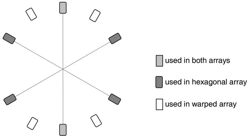
Regular hexagonal and warped hexagonal loudspeaker array with 2-meter radius
