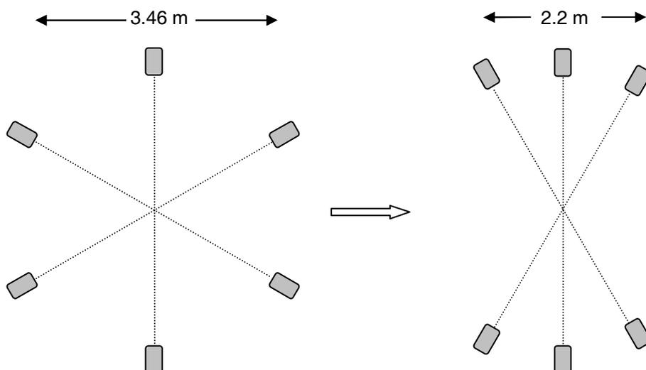
Fig. nn: Comparison of regular hexagonal and “warped” hexagonal loudspeaker arrays
