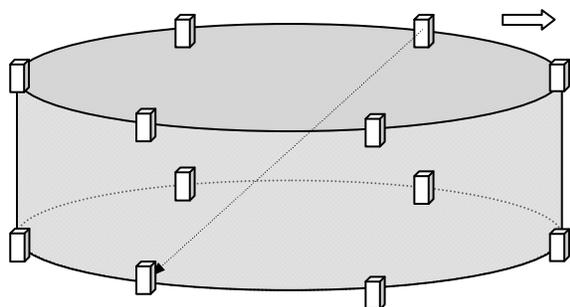
Figure nn: Cylindrical loudspeaker array.
