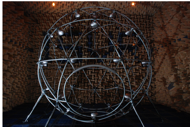
Figure 6: Picture of the loudspeaker array in the anechoic chamber of the ISVR.
