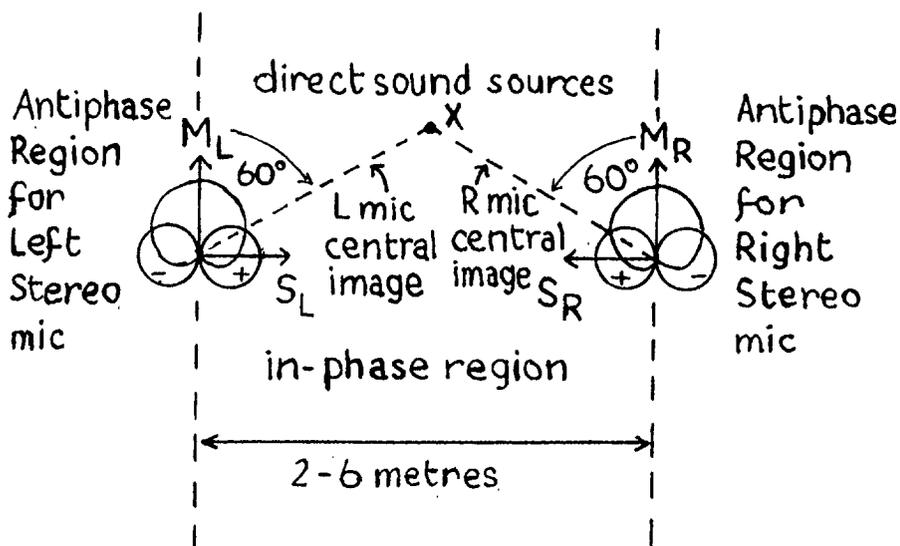
Figure 9. The use of a spaced pair of one-point stereo microphones, each of which is asymmetric, to cover a broad direct-sound-source stage. The gains of the  $S_L$  and  $S_R$  figure-of-eight microphones should ideally be such that a central sound source  $X$  in the stage is picked up as a central image, with equal channel gains, by both stereo microphones. Adapted from ref. [22].
