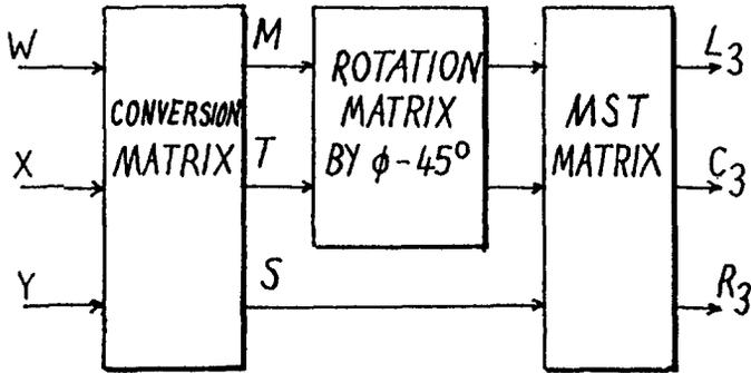
Figure 16. Use of frequency-dependent rotation matrix by angle  $\phi - 45^\circ$  in the M and T signal paths in the decoder of fig. 15. Typically,  $\phi = 35^\circ$  below 5 kHz and  $55^\circ$  above 5 kHz.
