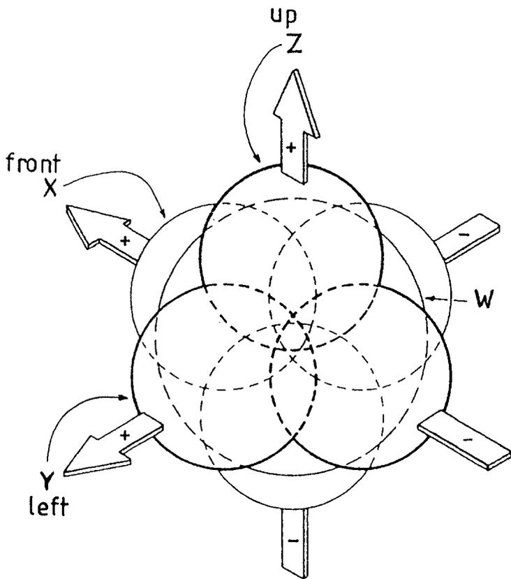
Figure 11. Polar diagrams of the B-format signals W (omnidirectional) and X, Y, Z (figure-of-eight with peak gain  $\sqrt{2} = 1.4142$ ) in 3 dimensions.
