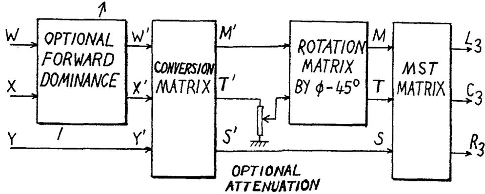
Figure 18. 3-loudspeaker decoder for B-format, showing T-channel gain adjustment before the frequency-dependent rotation matrix and forward dominance adjustment of the B-format input.
