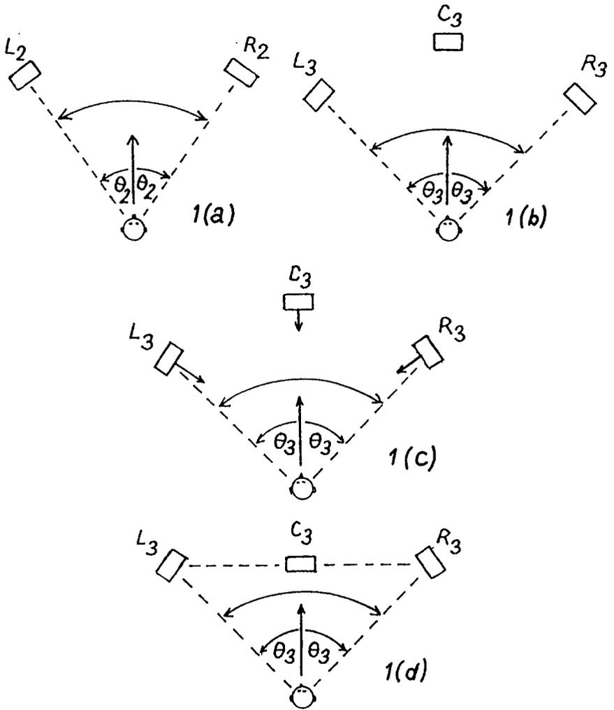
Figure 1. Two- and three-loudspeaker stereo layouts. 1(a) two loudspeakers. 1(b)-1(d) three loudspeakers. 1(a)-1(c) loudspeakers equidistant from ideally situated listener. 1(c) & 1(d) toed-in outer loudspeakers.
