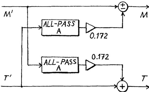
Figure 17. Implementation of a frequency-dependent rotation matrix for the decoder of fig. 16 using identical first-order all-pass networks with gain  $-1$  below 5 kHz and  $+1$  above.
