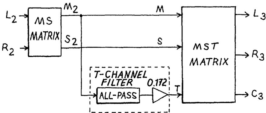
Figure 12. Psychoacoustically optimized  $3 \times 2$  decoder of fig. 7 implemented as an MST decoder with a synthetic T channel produced by filtering the M signal; adapted from fig. 14 of ref. [28].
