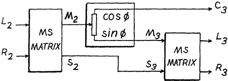
Figure 6. Form of  $3 \times 2$  decoder for three-loudspeaker reproduction of two-channel stereo using sine and cosine gains dependent on an angle parameter  $\phi$ .
