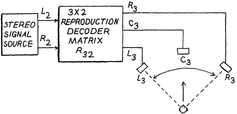
Figure 5. The reproduction of a 2-channel stereo source via three loudspeakers, using a  $3 \times 2$  psychoacoustic decoder.
