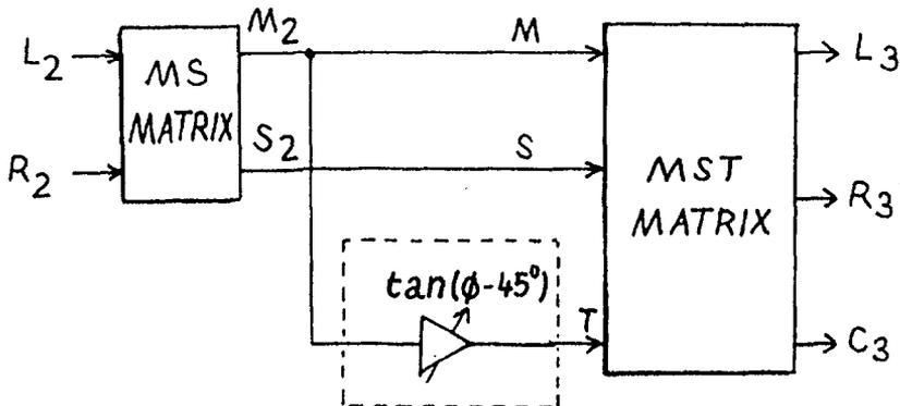
Figure 13. Version of the  $3 \times 2$  decoder of fig. 6 implemented in MST form using a synthetic T channel; this is only an approximation to the results of fig. 6, but the approximation is very good for  $|\phi - 45^\circ| \leq 15^\circ$
