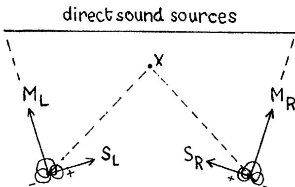
Figure 10. Illustrating the "splaying out" of the two stereo microphones, with  $M_L$  and  $M_R$  pointing at the edges of the stage, for a sound stage wider than the microphone spacing.
