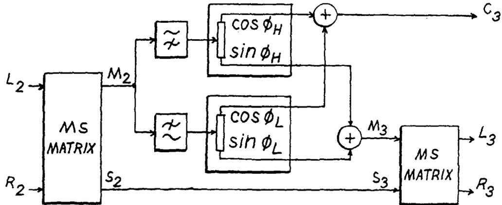
Figure 7. Frequency-dependent version of the  $3 \times 2$  decoder of fig. 6, using low and high pass filters preceding different values,  $\phi_L$  and  $\phi_H$ , of the decoder parameter  $\phi$  at respective lower and higher frequencies around 5 kHz. Recommended values are  $\phi_L = 35.26^\circ$  and  $\phi_H = 54.74^\circ$ .
