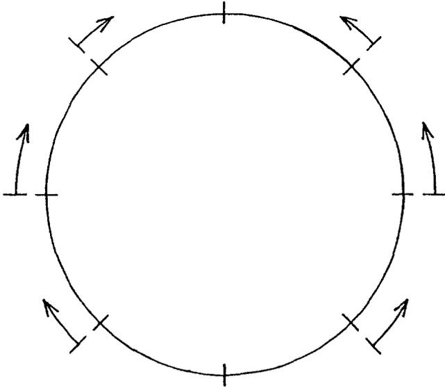
Figure 19. The effect of  $\lambda = \sqrt{2}$  forward dominance on the encoded azimuths of B-format signals in the horizontal plane.
