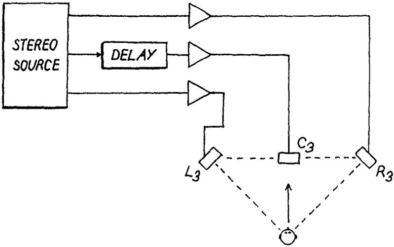
Figure 2. Use of time delay to compensate for unequal distances of loudspeakers from an ideally-situated listener.
