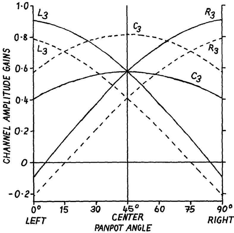
Figure 8. Channel gains for three loudspeakers  $L_3$ ,  $C_3$ ,  $R_3$  when a constant-power sine-cosine two-channel panpot is fed to a psychoacoustically-optimized  $3 \times 2$  decoder. Chained lines: low frequencies below 5 kHz, with  $\phi = 35.26^\circ$ ; solid lines: high frequencies above 5 kHz, with  $\phi = 54.74^\circ$ .
