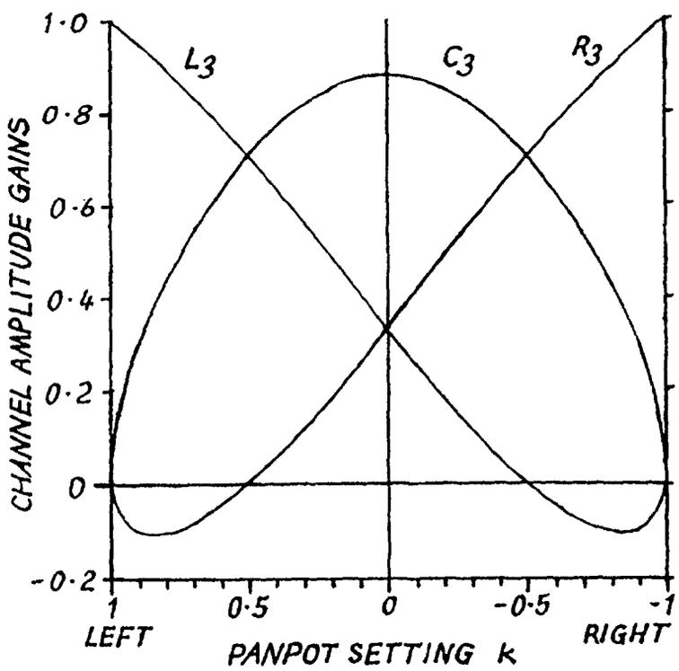
Figure 3. "Optimum" 3-channel panpot law gains for 3-loudspeaker stereo feeds  $L_3$ ,  $C_3$  and  $R_3$ , ensuring consistency of different localization cues and minimizing geometric image distortions for noncentral listeners.
