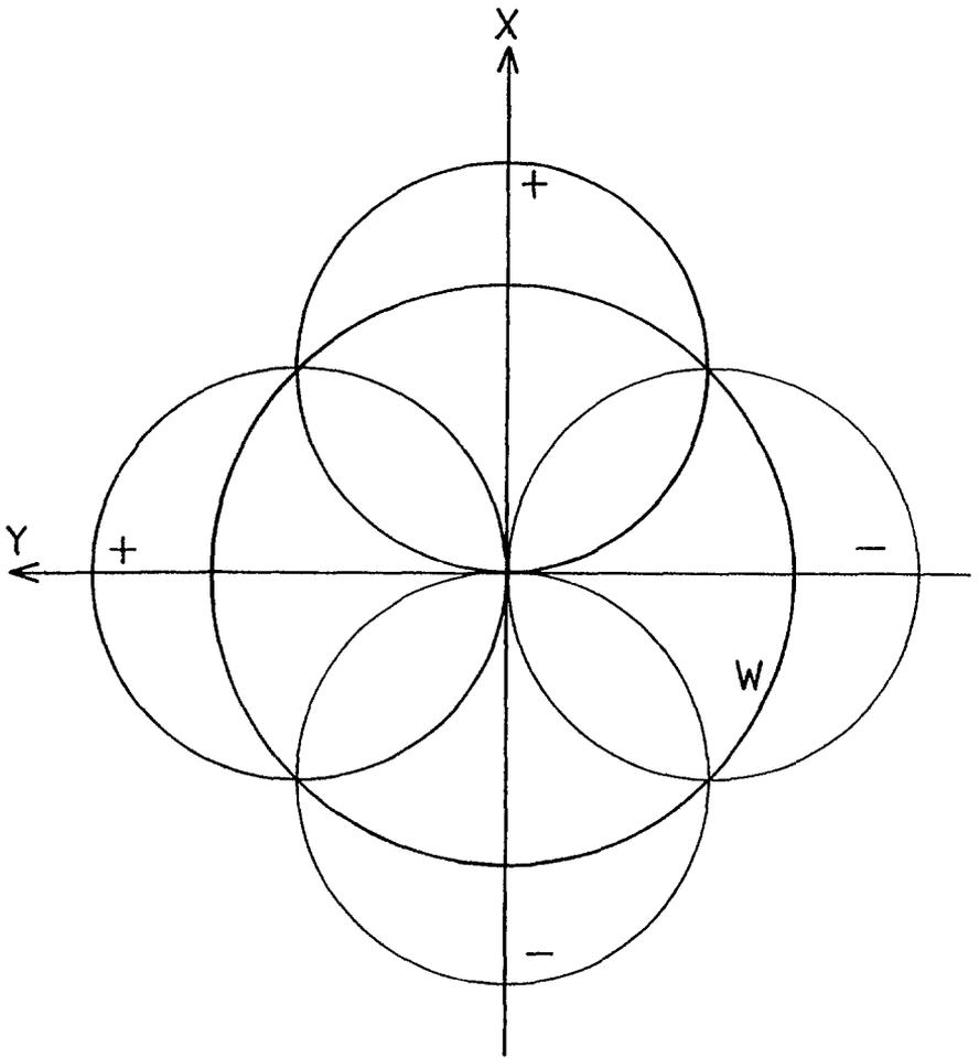
Figure 14. B-format directional polar diagrams in the horizontal plane as a function of azimuth angle.
