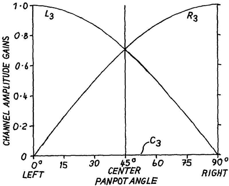
Figure 4. Channel gains for conventional sine/cosine constant-power sine-cosine panpot law for two-loudspeaker stereo, fed to three loudspeakers; the center loudspeaker  $C_3$  gain is zero.
