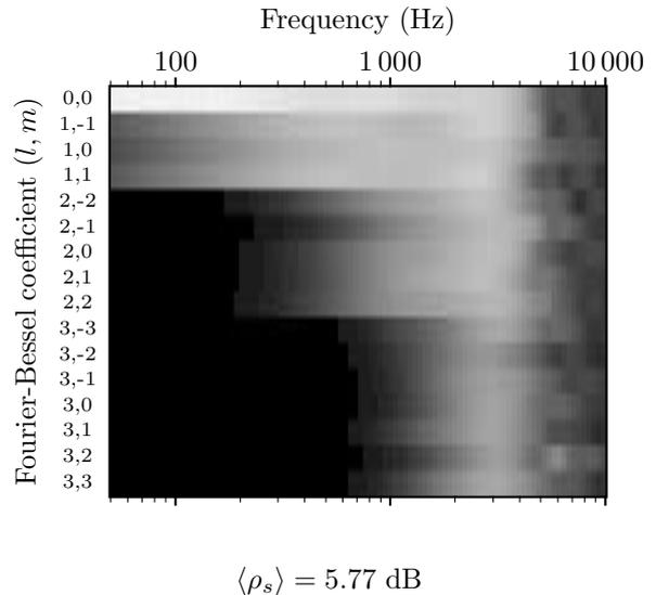
Fig. 21: Spatial signal to noise ratio for our prototype.
