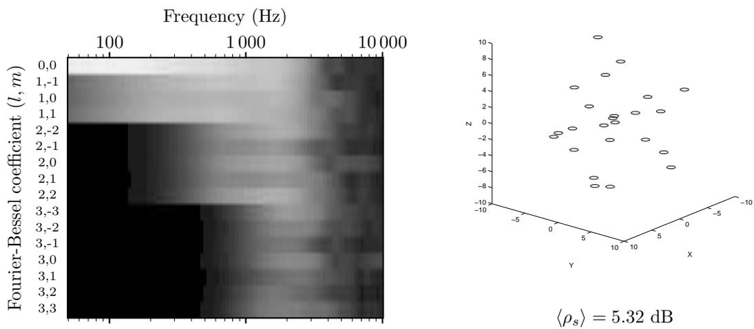
Fig. 15: Spatial signal to noise ratio for a full three dimensional microphone array.
