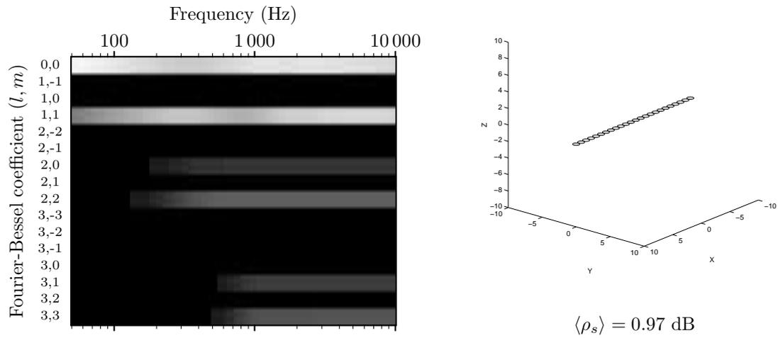
Fig. 12: Spatial signal to noise ratio for a linear microphone array.
