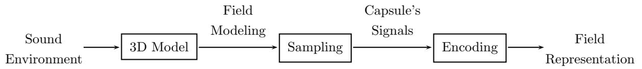
Fig. 1: Principle diagram.
