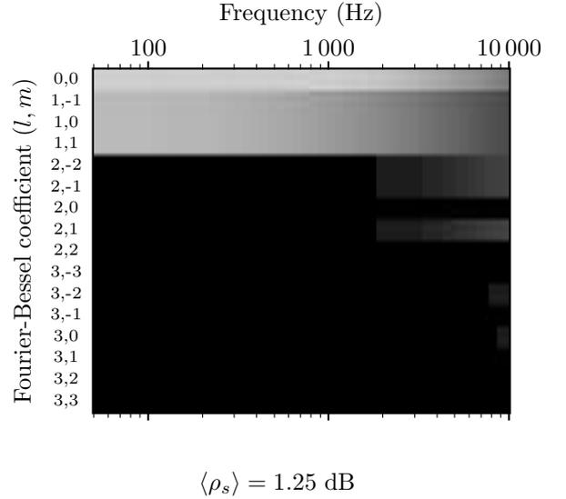
Fig. 18: Spatial signal to noise ratio for a SoundField microphone.
