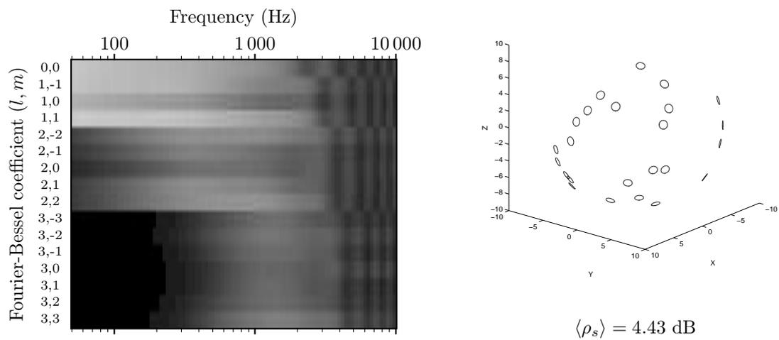
Fig. 17: Spatial signal to noise ratio for a spherical microphone array with cardioid capsules.
