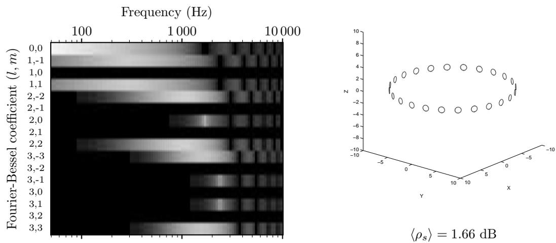
Fig. 13: Spatial signal to noise ratio for a circular microphone array.
