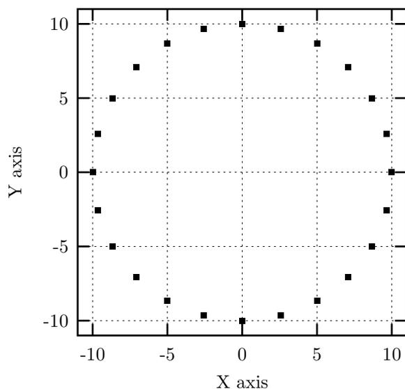
Fig. 9: Layout of the circular microphone array.
